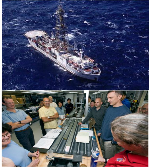
Photo (top): JOIDES Resolution (deep-sea drilling vessel), Photo (bottom): Strata drilled from the seabed (deep-sea sediment core)
