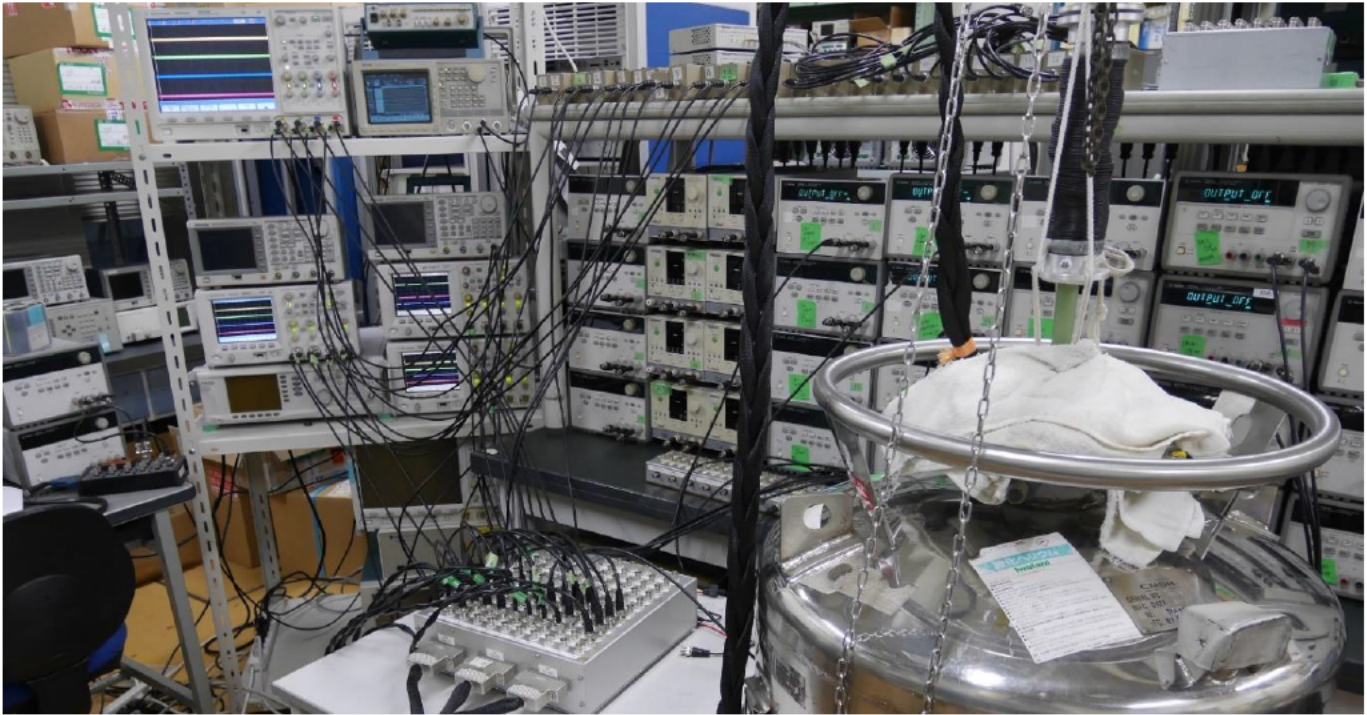
Photo: Facility for evaluating the superconducting circuit. The circuit is submerged in liquid helium at -269^{\circ}\text{C} from a storage vessel (lower right of the photograph) to maintain the superconducting state, to measure its electric characteristics and circuit response.
