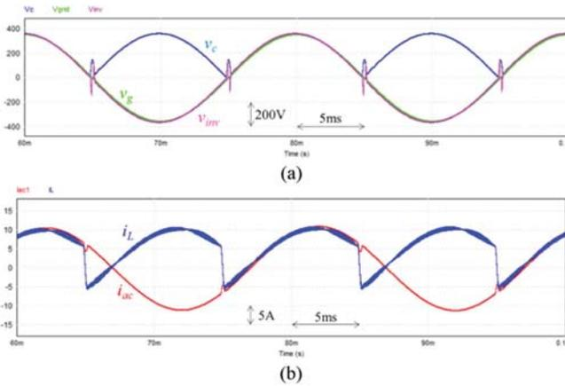
**FIGURE 35. Simulation result in the steady-state: (a) Capacitor voltage  $v_c$ , grid voltage  $v_g$ , and inverter voltage  $v_{inv}$ ; (b) dc inductor current  $i_L$ , and ac current  $i_{ac}$ .**
