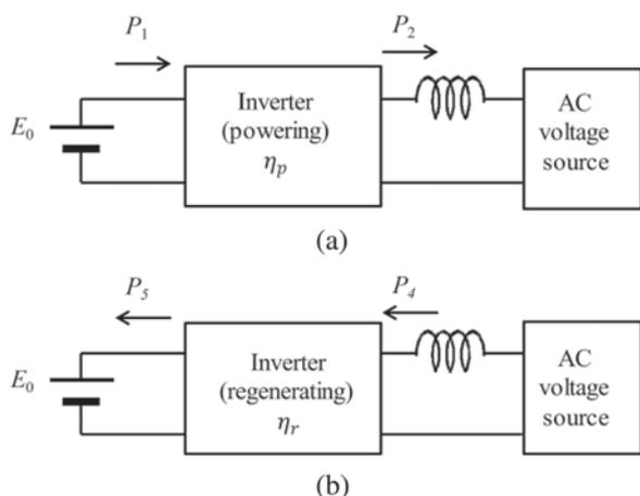
Fig. 4. Basic structure of virtual transformer-based BTB asynchronous loss measurement method using one set of measurement instruments (VTASLM) [19]. (a) Powering power measurement and (b) Regenerating power measurement
