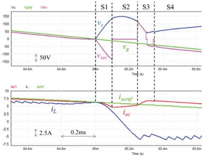
**FIGURE 27.** Zoomed-in waveforms near the voltage zero crossing.
