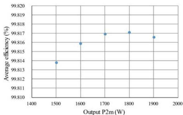
Fig. 11. Measured average efficiency of GaN HEECS inverter by VTASLM [19]
