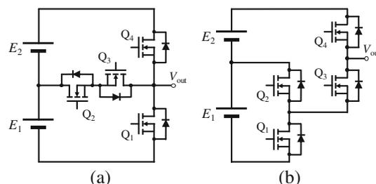
Fig. 13. T-type and HEECS circuit topology [37]. (a) T-type and (b) HEECS
