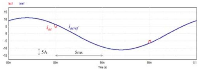
**FIGURE 37. Simulation result: Ac current reference  $i_{acref}$  and ac current  $i_{ac}$ .**
