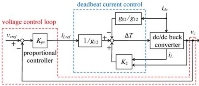
**FIGURE 6.** Control block diagram of DBCCL + VC.
