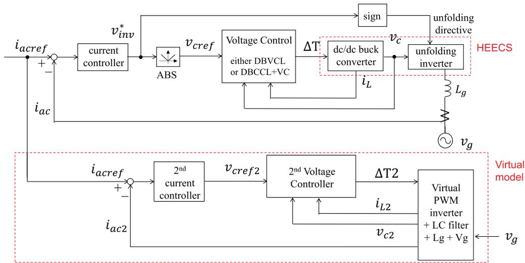
FIGURE 23. Control block diagram including both the real model and virtual model.
