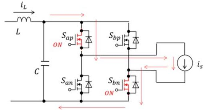
**FIGURE 10.** Current path before voltage zero crossing in the lagging PF mode.
