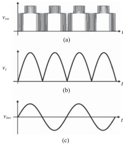
**FIGURE 3.** Voltage waveforms of the HE ECS: (a) dc/dc converter switching circuit output voltage, (b) dc capacitor voltage, (c) inverter output voltage.
