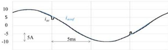
FIGURE 40. Experimental results: Zoomed-in ac current (in black) and ac current reference (in blue).
