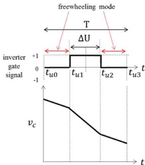
FIGURE 17. Waveforms in the reverse-polarity PWM mode.
