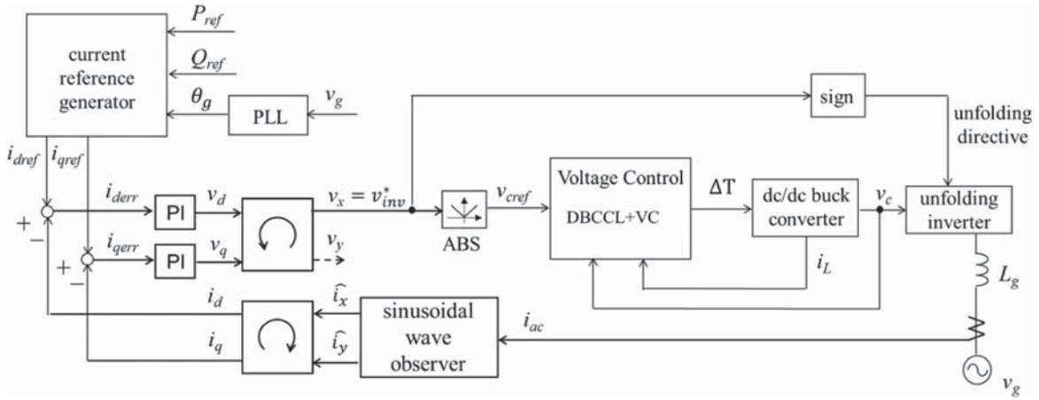
**FIGURE 46.** Control block diagram of current control for the grid-connected inverter based on HEECS.
