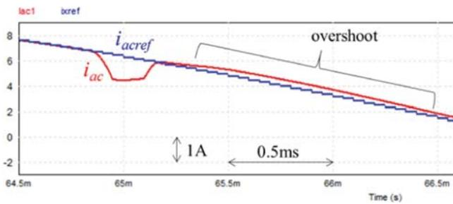
FIGURE 29. AC current waveform with three-cycle forward unfolding timing.
