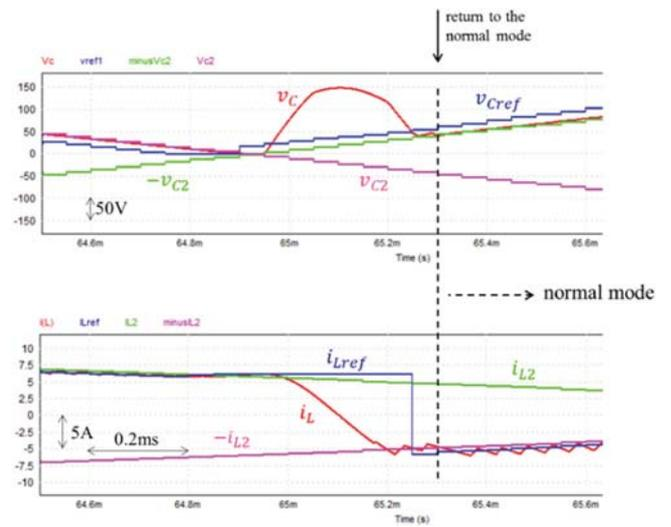
FIGURE 25. Simulation result when the target values are determined from the virtual circuit.
