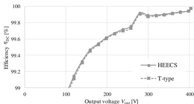
Fig. 14. Comparison of efficiency between T-type and HEECS [37]
