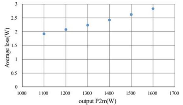
Fig. 8. Measured average loss of SiC-HEECS inverter by VTASLM [19]
