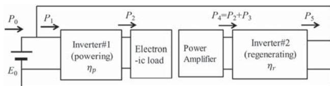
Fig. 3. A BTB loss measurement system based on virtual ideal transformer [19,25]
