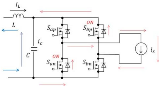
FIGURE 16. Current path of the regular-polarity PWM mode in Section S3.
