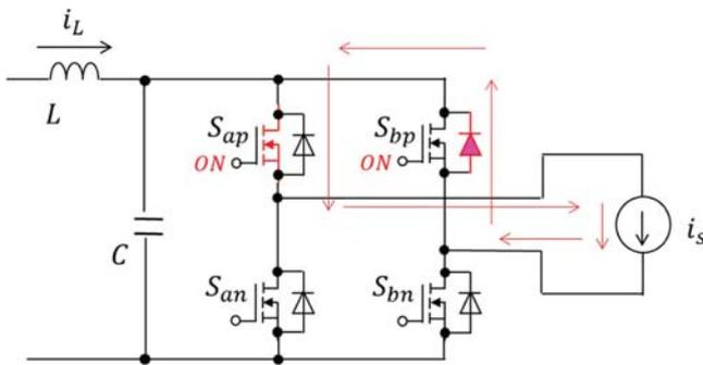
**FIGURE 13.** Freewheeling mode for Section S2.
