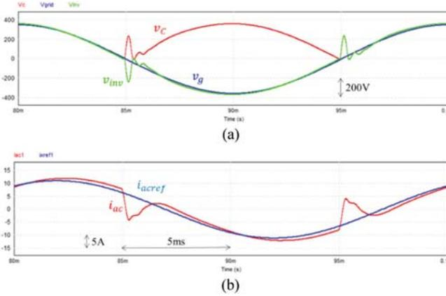
**FIGURE 7.** Simulation waveforms of an HECS controlled by DBCCL + VC in lagging PF operation (a) dc capacitor voltage  $v_c$ , inverter output voltage  $v_{inv}$ , and grid voltage  $v_g$ , (b) grid current reference  $i_{acref}$ , and grid current  $i_{ac}$ .
