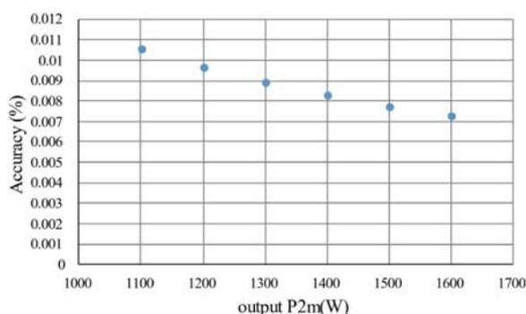
Fig. 10. Accuracy of SiC-HEECS inverter efficiency measurement by VTASLM
