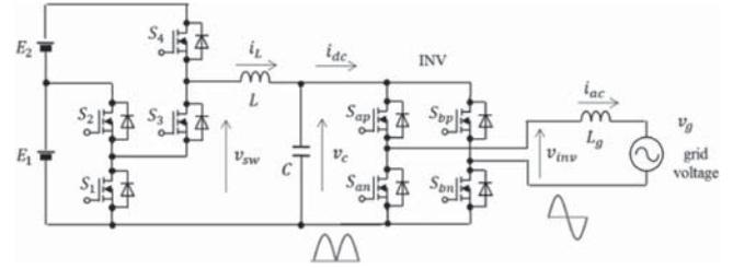
**FIGURE 2.** Grid-connected inverter based on the HEECS.
