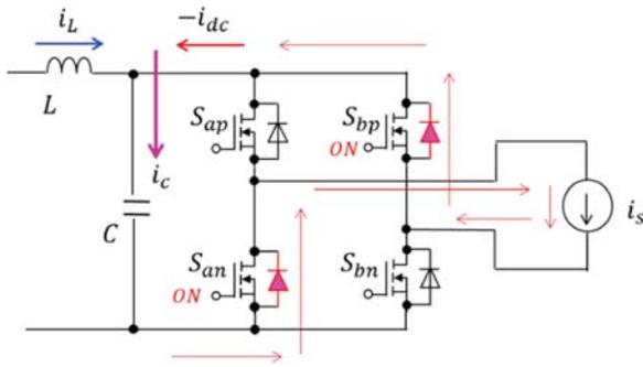
**FIGURE 11.** Current path just after voltage zero crossing in the lagging PF mode.
