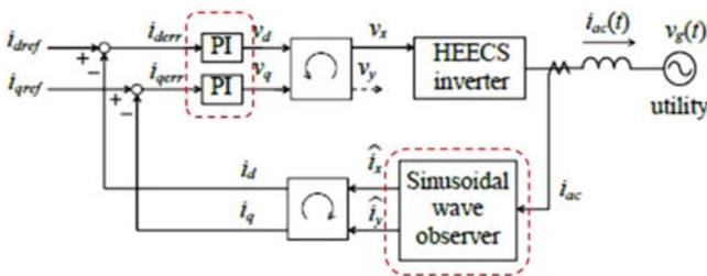
FIGURE 30. Current control block diagram.
