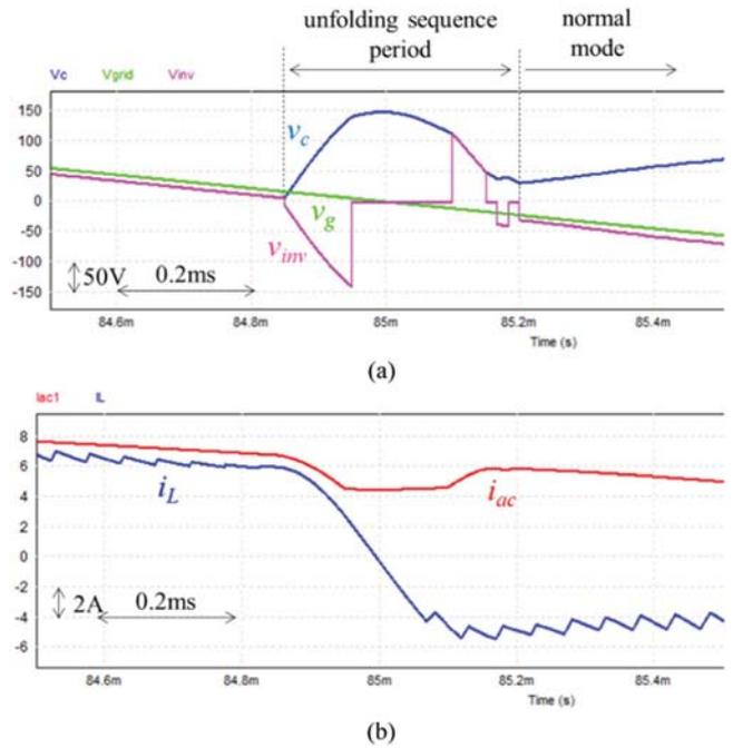
**FIGURE 36. Simulation result: Zoomed-in waveforms near unfolding: (a) Capacitor voltage  $v_c$ , grid voltage  $v_g$ , and inverter voltage  $v_{inv}$ ; (b) dc inductor current  $i_L$  and ac current  $i_{ac}$ .**
