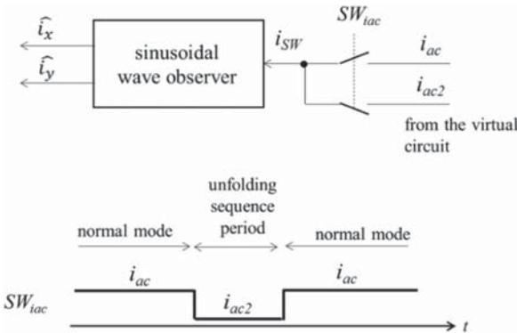
FIGURE 31. AC current signal selection to the sinusoidal wave observer in Fig. 30.
