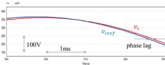
**FIGURE 21.** Simulation example: dynamics between  $v_{cref}$  and  $v_c$ . (Conditions are the same as those for Fig. 20).
