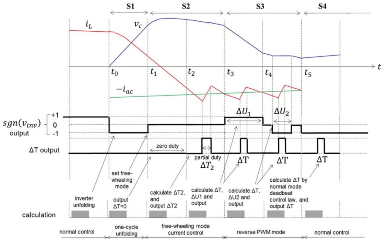
**FIGURE 12.** Timing chart after voltage zero crossing.
