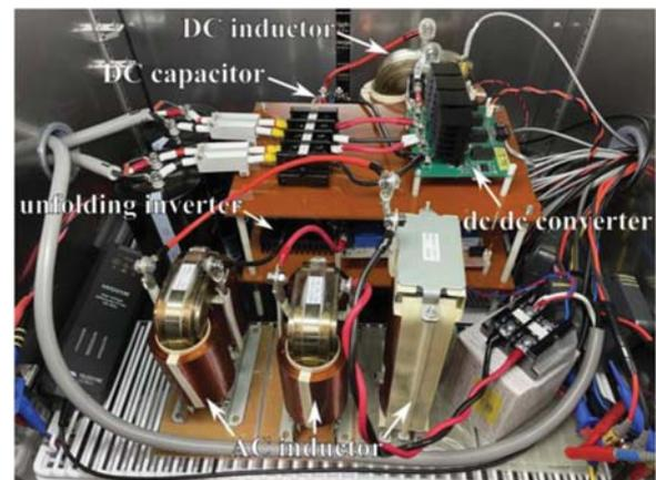
FIGURE 34. Circuit under test.
