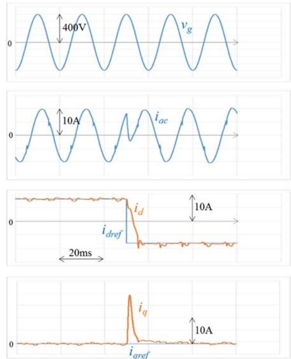
FIGURE 43. Experimental results: Transient response.
