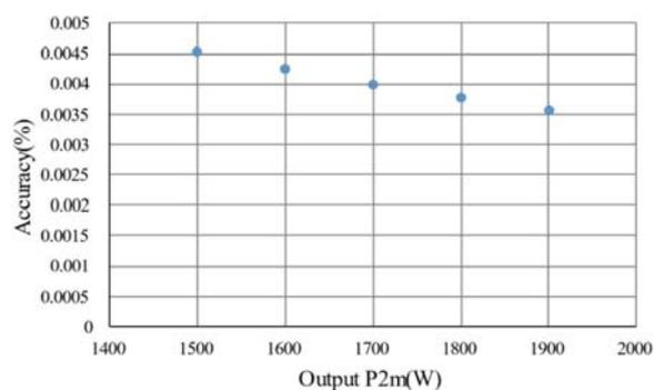
Fig. 12. Accuracy of GaN-HEECS inverter efficiency measurement by VTASLM
