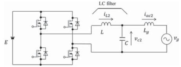
**FIGURE 22.** Circuit diagram of the proposed virtual PWM inverter.
