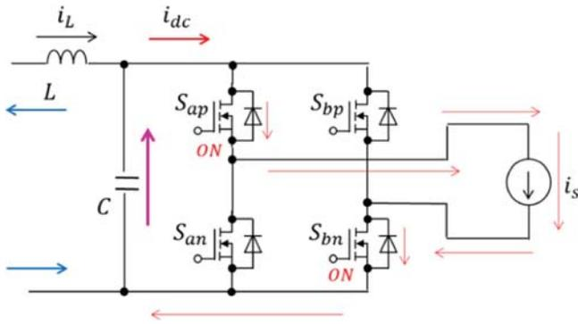
FIGURE 15. Current path of the reverse-polarity PWM mode in Section S3.
