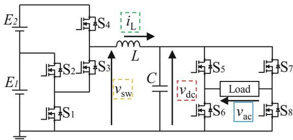
Fig. 1. Two battery HEECS inverter [4,5]
