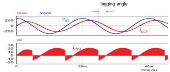
**FIGURE 9.** Simulated waveforms of the conventional PWM grid-connected voltage source inverter in lagging PF operation.
