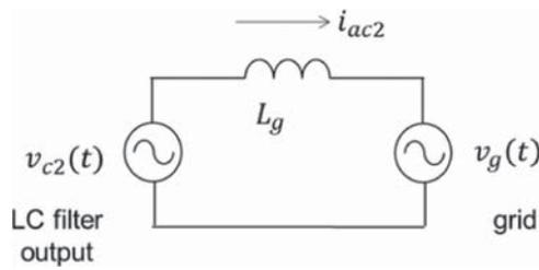
FIGURE 24. Circuit diagram of the virtual grid-tie circuit.
