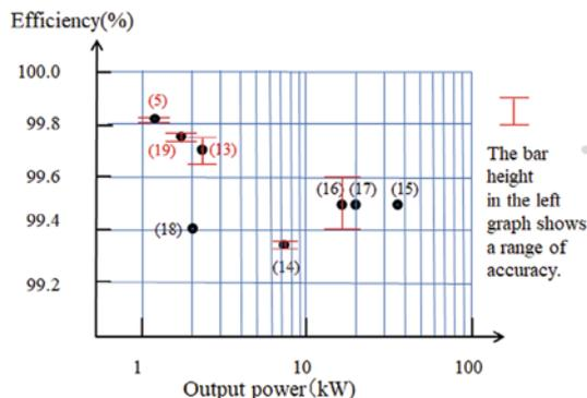
Fig. 2. Survey of high efficiency inverters [5]
