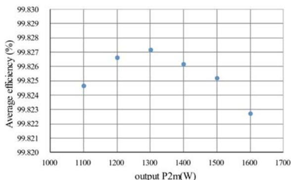
Fig. 9. Measured average efficiency of SiC-HEECS inverter by VTASLM [19]
