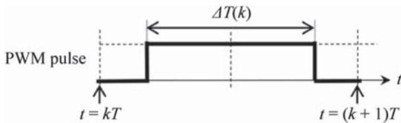
**FIGURE 5.** PWM pulse waveform.
