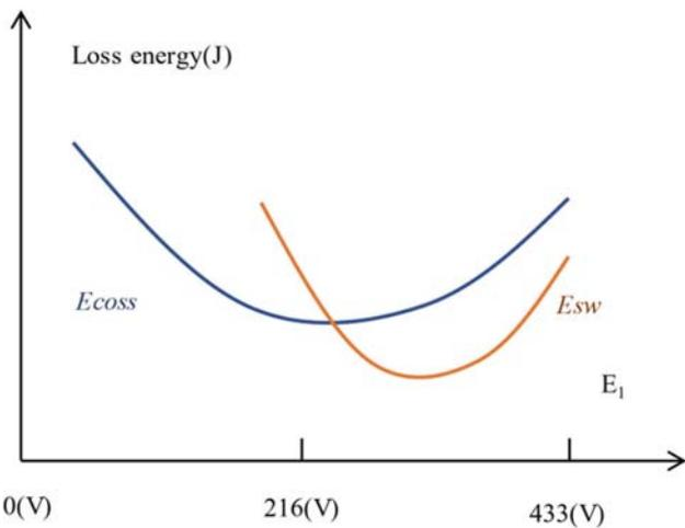
Fig. 6. Qualitative illustration on loss of  $C_{oss}$  and switching regarding  $E_1$  ( $(E_1 + E_2)/2 = 216.5(V)$ )
