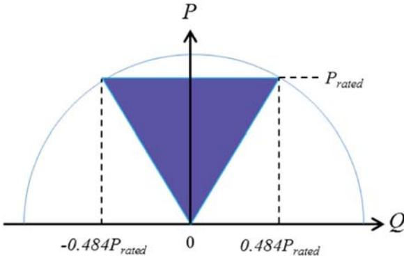
**FIGURE 1.** Reactive power requirements for distributed energy resources [19].
