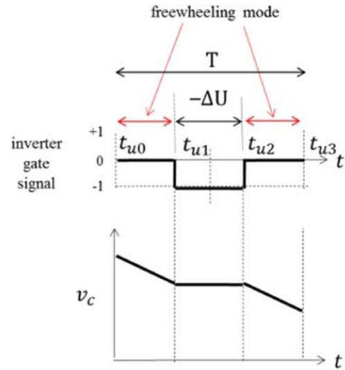
FIGURE 18. Waveforms in the regular-polarity PWM mode.
