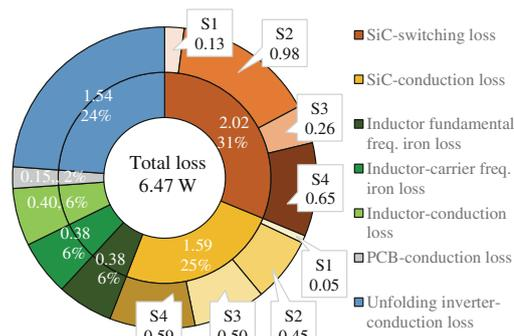
Fig. 5. Loss breakdown ratio of DC-AC conversion (2.2 kW) of SiC-HEECS inverter (symbols S1, S2, S3, and S4 are the same as those in Fig. 1) [13]
