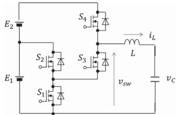
**FIGURE 14.** Equivalent circuit of the dc/dc converter during Section S2.
